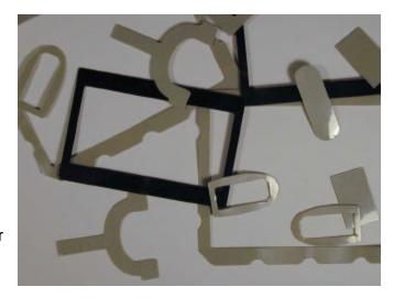
window gaskets. This silicone rubber composite has been specified for hand held and portable units requiring extreme low temperature functionality. The 30 durometer silicone rubber substrate with silicone polymer adhesive on both sides allows for thermal expansion and contraction of mating plastic components and metal frames and maintains consistent bond strength down to -70°F.
