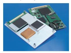
Gap Pad® 1500 has an ideal filler blend that gives it a low-modulus characteristic that maintains optimal thermal performance yet still allows for easy handling. The natural tack on both sides of the material allows for good compliance to adjacent surfaces of components, minimizing interfacial resistance.
