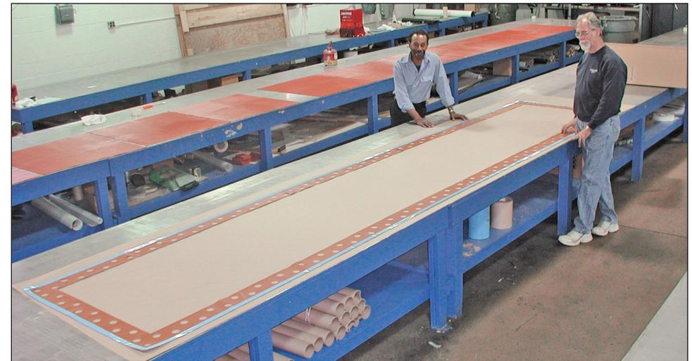
**Jim Pelzer (left) and Jay Hough show off one of Stockwell's product lines: fabricated silicone sponge gaskets for radomes—dome-like covers for radar units—which are water-jet cut and spliced together using ultraviolet-cured silicone adhesives.**
