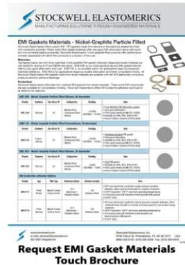
Stockwell Elastomerics' nickel-plated graphite filled compounds (<http://www.stockwell.com/emi-shielding-materials.php>) have been third party tested for shielding effectiveness per Mil-G-83528 standards. With very good attenuations properties, these compounds are often selected for defense applications and commercial applications where silver-plated aluminum compounds are too costly.
