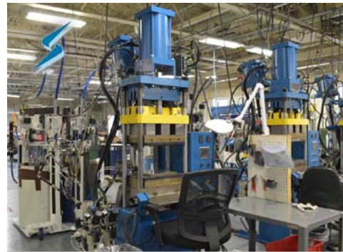
New liquid injection molding machines at Stockwell Elastomerics
